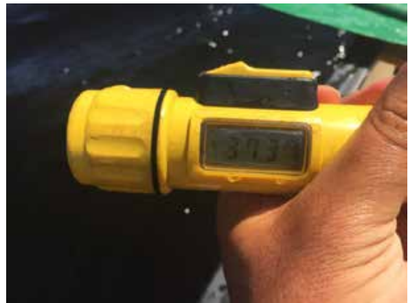
Figure 1. Depth sounder utilized to determine the extent of the littoral zone as well as the location of the deep hole where plankton tows were deployed. The digital display reads 37.3ft, too deep for aquatic plants.
